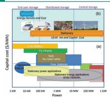
The different applications of energy storage, different technologies, and the cost requirements from the kilowatt to gigawatt scale are compared. Li-ion batteries have attracted attention for transportation storage, while many other technologies are considered for stationary applications.
