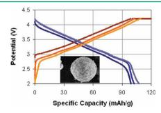
The research and development of ambient temperature Na-ion batteries is progressing quickly and is now poised to penetrate the energy storage landscape. The combination of new electrode materials, electrochemical couples, and engineering advances coupled with a potential for low-cost and long-life make them attractive candidates for grid storage.
