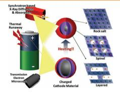
The structural origin of the thermal instability of cathode materials, which is a critical safety issue for lithium-ion batteries, is studied systematically using a combination of various in situ synchrotron X-ray techniques and transmission electron microscopy. The in-depth understanding of the thermal decomposition behavior of overcharged cathode materials provides valuable guidance for developing new cathode materials with improved safety characteristics.
